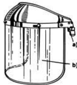
Class 6A Face shield for impact, piercing, splash, head, and glare protection. a) hard hat attachment; b) face shield (window).
